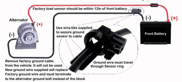
Your factory ground sensor wire must be removed and replaced with the new upgraded black ground wire we supply in the kit
